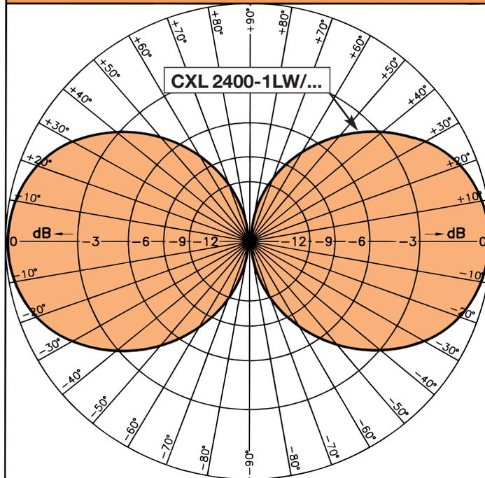
**TYP. STRAHLUNGSDIAGRAMM (HORIZONTAL)**
